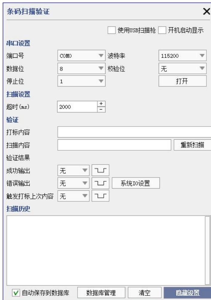
The image shows a software dialog box titled "条码扫描验证" (Barcode Scanning Verification). It contains several sections for configuration and operation:
